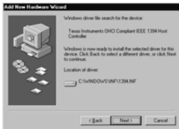
5. When Windows has finished copying and installing the device drivers, it will display the following dialog box. Click "Finish" to complete installing the FireHost adapter.
