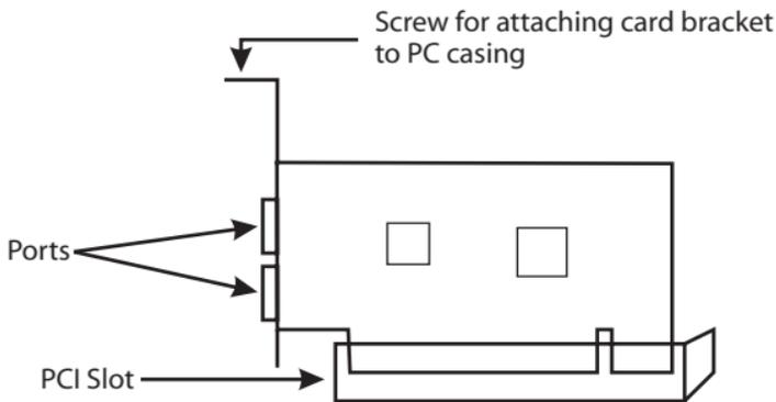
4. Unscrew and remove the metal slot cover corresponding to the slot that will hold the FireHost card, and retain the screw.
