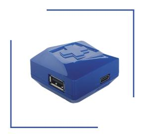
The small adapter can easily be carried around in your pocket and it features an OTG mode. Like with SimulCharge<sup>™</sup>, the mobile device remains as USB Host so it can communicate with peripherals. However, unlike SimulCharge<sup>™</sup>, OTG mode lets the mobile device to power the peripherals from its own battery. This allows you to use the Charge-Plus without an external AC power source.
